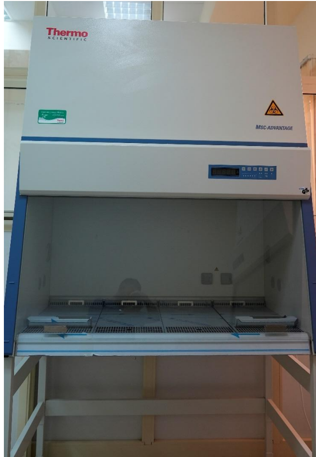
1. laminar flow hood [ SG403A-HE-INT]
